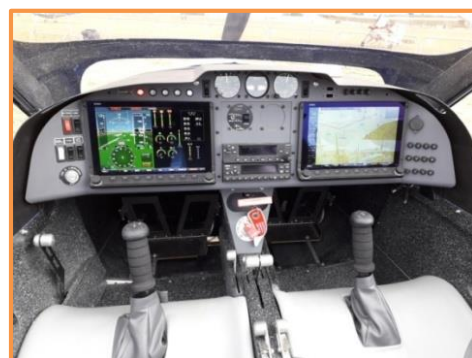
Instrument panel: Double SkyView HDX Dynon Avionics (option)
